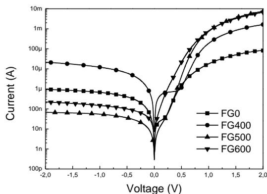
**Fig. 2:** Dark  $I$ - $V$  curves of samples annealed in the forming gas.
