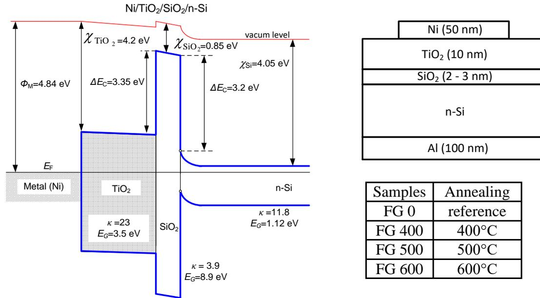
**Fig. 1:** Band diagram of the Ni/TiO<sub>2</sub>/SiO<sub>2</sub>/n-Si structure, cross-sectional view of the structure and sample labelling.
