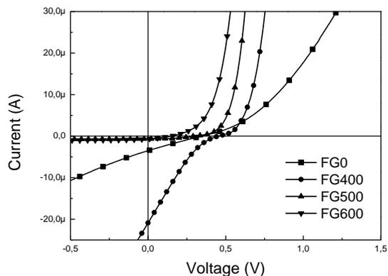
**Fig. 3:** Light  $I$ - $V$  curves of samples annealed in the forming gas.
